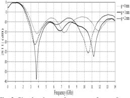
Fig. 2. Simulated return loss curves for g = 0 mm, g = 1 mm and g = 2 mm.
