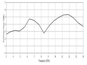
Fig. 7. Gain of the antenna.
