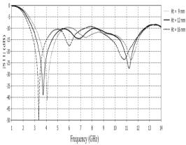
Fig. 3. Simulated return loss curves for  $H_t = 9$  mm,  $H_t = 12$  mm and  $H_t = 16$  mm.
