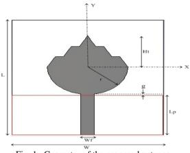
Fig. 1. Geometry of the proposed antenna.
